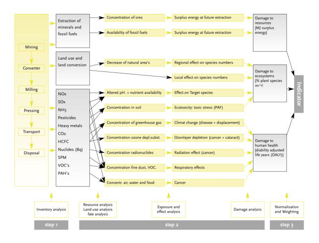
Figure 7: Detailed representation of the damage model (step 2)
