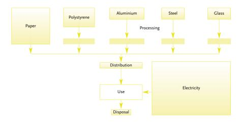
Figure 4: The coffee machine process tree, where the size of the process blocks is proportional to the relative importance of the process.
