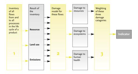
Figure 6: General procedure for the calculation of Eco-indicators. The light coloured boxes refer to procedures, the dark coloured boxes refer to intermediate results.
